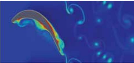
▲ **External compressible aerodynamics:** modelling flow separation over a turbine blade.
