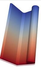
Axial displacement test of an Embraer aircraft stiffener.
